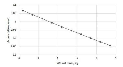
Fig. 5. Acceleration vs. individual wheel mass
