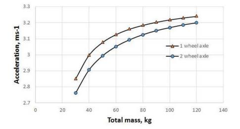
Fig. 4. Acceleration vs. total vehicle mass
