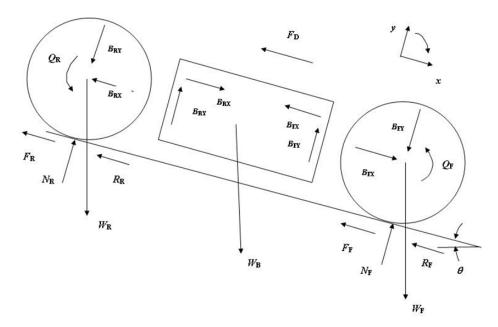
Fig. 3. Free body diagrams of a gravity propelled vehicle
