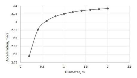
Fig. 6. Acceleration vs. wheel diameter
