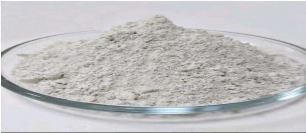
Fig. 3. Calcinated and grounded Cow Bone Ash (CBA)
