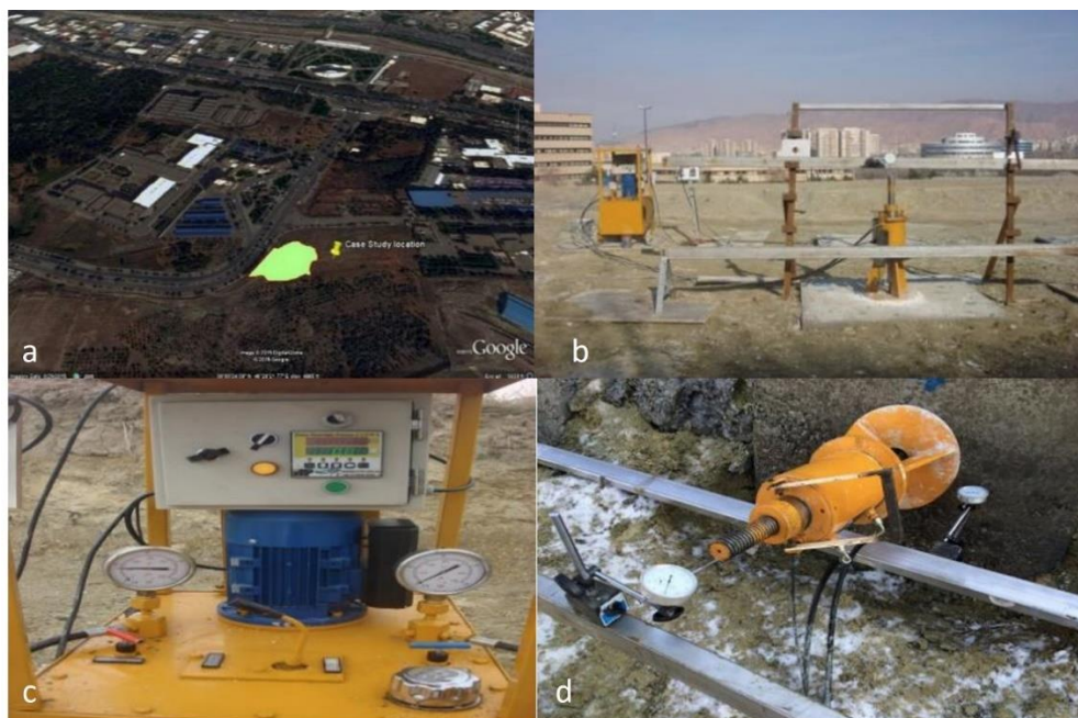
Fig. 1. Aerial image of the study site along with the tension-compression jack and its peripherals. (a) areal images of the study site. (b) The jack system and its accessories installed at the study site. (c) Data logging and pressure calibration device. (d) The interface connecting the jack to the anchor and installation of measurement gauges. Axial displacement of the anchor and the concrete pad settlement
