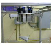
Figure 12. Cable-suspended robot designed and assembled at University of Delaware [20].
