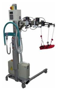
Figure 19. MariBot—a platform for upper arms using cable-based parallel manipulator [28].
