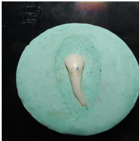
Fig. 1. Specimen Mounted in Dental Stone
