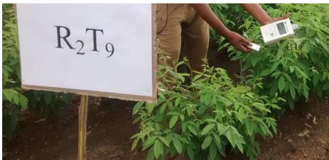
Fig. 2. Leaf Porometer (SC-1 porometer, Decagon Devices, Pullman, WA, USA) used during the experiment
