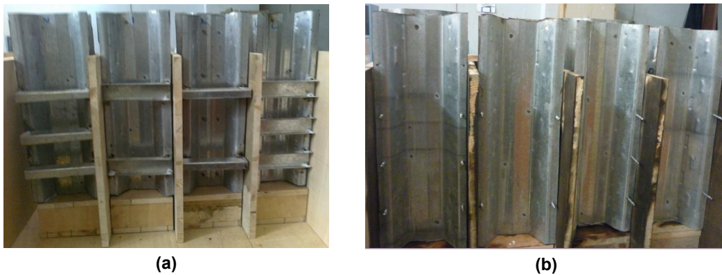
Fig. 4. Specimens enhanced with cold formed members (U, C) (a) and enhanced with Self-drilling screws (b)
