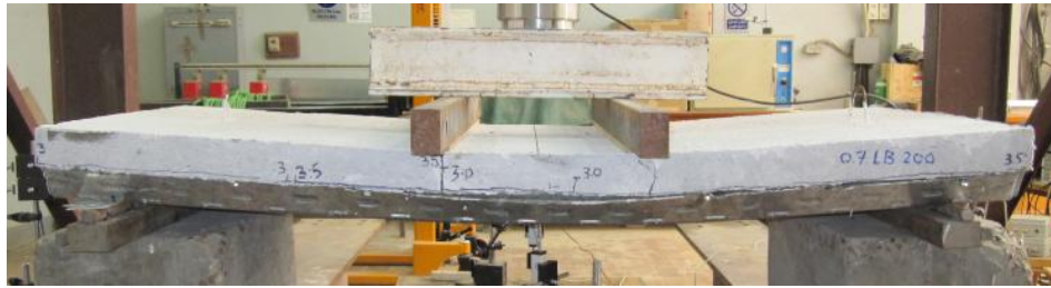
Fig. 14. Crack pattern for tested specimen (0.7 LS 200)
