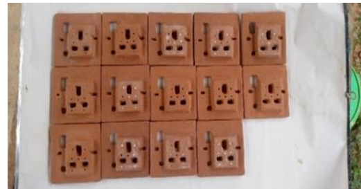
Fig. 11. Fired Samples of the Socket
