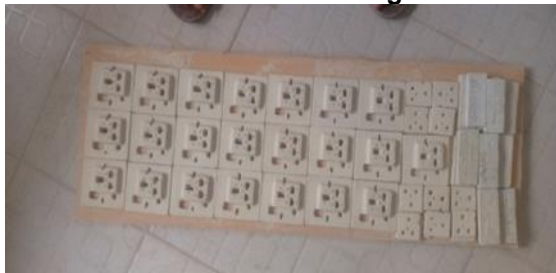
Fig. 10. Fired Samples of the Socket
