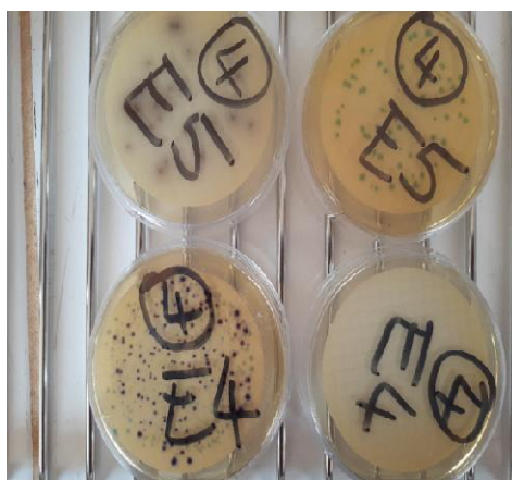
Fig. 2. Faecal coliforms (blues) and E. coli (violet) on chromogenic rapid E. coli 2 agar
