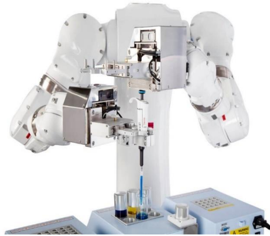
Fig. 10. Two-arm MOTOMAN CSDA10F robot
