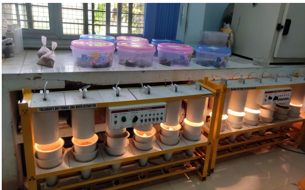
Plate 2. Setting of berlese funnel for the estimation of soil invertebrate population from collected samples
