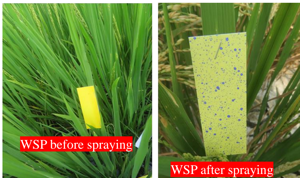
Fig. 3. Placement of water-sensitive paper to collect spray droplets for measuring droplet size
