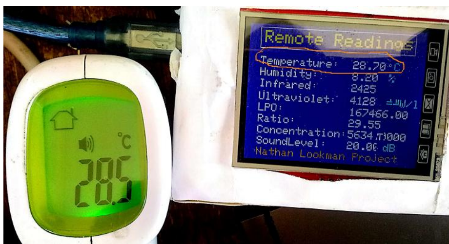
Fig. 5. Temperature reading of Infra-red thermometer compared with designed EC-DAQS
