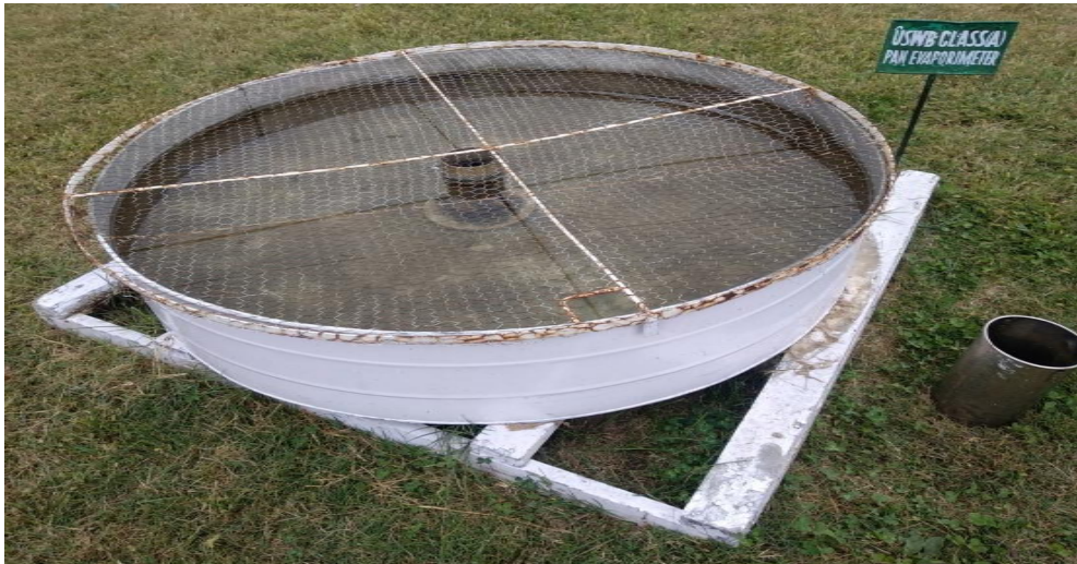
Fig. 3. USWB CLASS(A) Pan evaporimeter installed at agromet station of SKUAST-Kashmir
