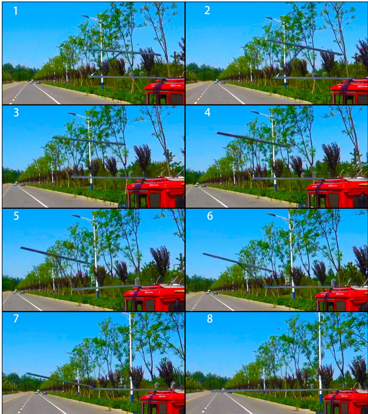
Figure 7. The unfolding process of the wings. 1–8 shows the process of morphing in chronological order.
