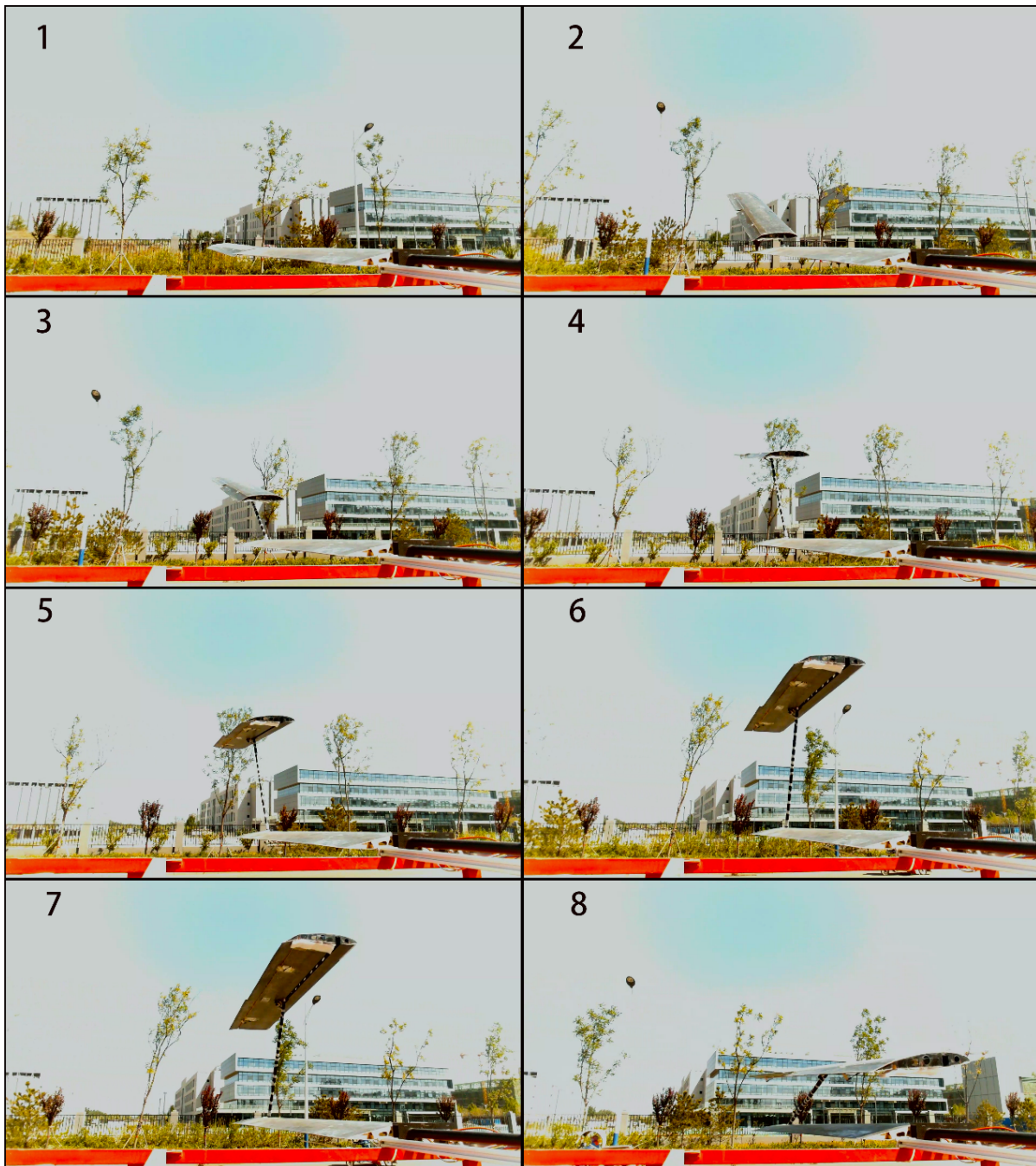
Figure 8. The folding process of the wings. 1–8 shows the process of morphing in chronological order.
