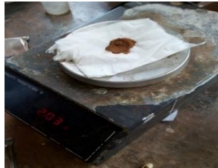
Fig. 1. Measurement of vitiated soil weight prior to extraction
