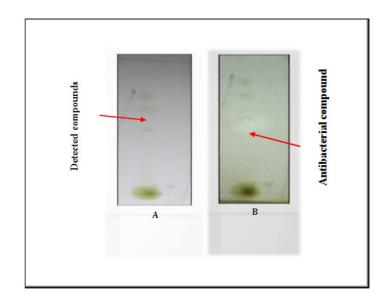
Fig. 2. (A-B). (A) Normal plate developed in solvent mixture benzene: acetone (9:1, v/v) showing the detected components under UV at 365 nm. (B) TLC-DB, developed in solvent mixture benzene: acetone (9:1, v/v) and viewed under UV at 365 nm showing the compound with the antibacterial activity
